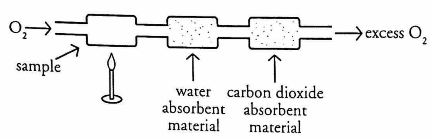
In a combustion analysis experiment, a hydrocarbon sample is heated in a stream of oxygen gas. As the sample burns, water and carbon dioxide is pushed through a series of chambers with materials that absorb each of the respective products. The chambers are each weighed before and after the combustion to determine the mass of each product.
